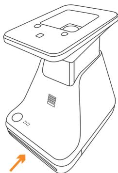
**04** **Close the film door.** The darkside will eject automatically beneath the film shield. Lift the film shield and allow it to roll back up, then remove the darkside.
