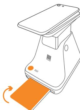
**08** **Your photo will eject beneath the film shield.** After five seconds, lift the film shield, allow it to retract into the Polaroid Lab and then gently remove your photo.
