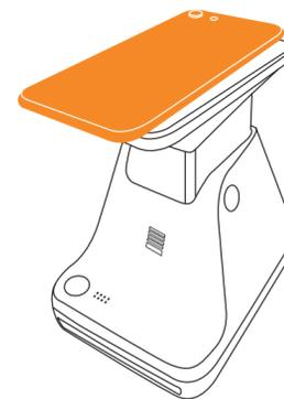
**06** Place your phone on the Polaroid Lab platform with the screen facing down. **Ensure that your phone is aligned lengthways and the top of your phone is facing the top of the platform.** Remove any screen protector or phone cover, as this can impair final results.
