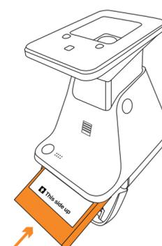
**03** Insert the film pack with the darkside cover facing up. **Use only Polaroid i-Type or Polaroid 600 type film.**
