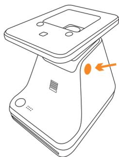
**01** Remove the cover from the platform. **Turn the Polaroid Lab on by pressing the platform release button on the right side of the Lab.** The phone platform will automatically lift into ready position. Check that the rainbow LED is lit up.
