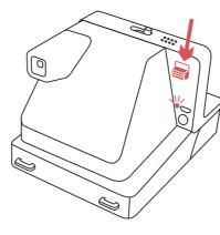
Turn the OneStep+ on by moving the **ON/OFF switch M** to the ON position, and check that the Flash LED (1) is green
