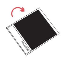
Don't shake or bend the photo! Shield it from light (in a pocket, or face down on a flat surface) until the image begins to emerge - black & white photos take 5-10 minutes, while color pictures take 10-15 minutes
