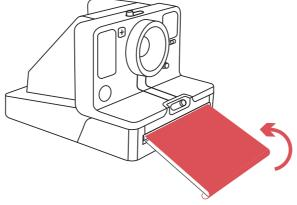
Your photo will eject beneath the film shield (1). After five seconds, lift the film shield, allow it to retract in the camera, then remove your photo
